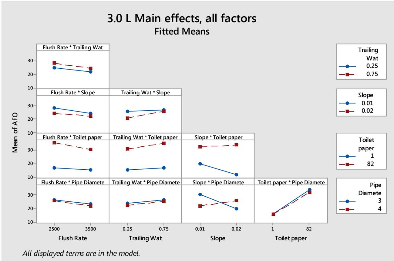
Table 4-12, General Linear Model: AFO versus Flush Rate, Trailing Water, Slope, Toilet paper, Pipe Diameter
