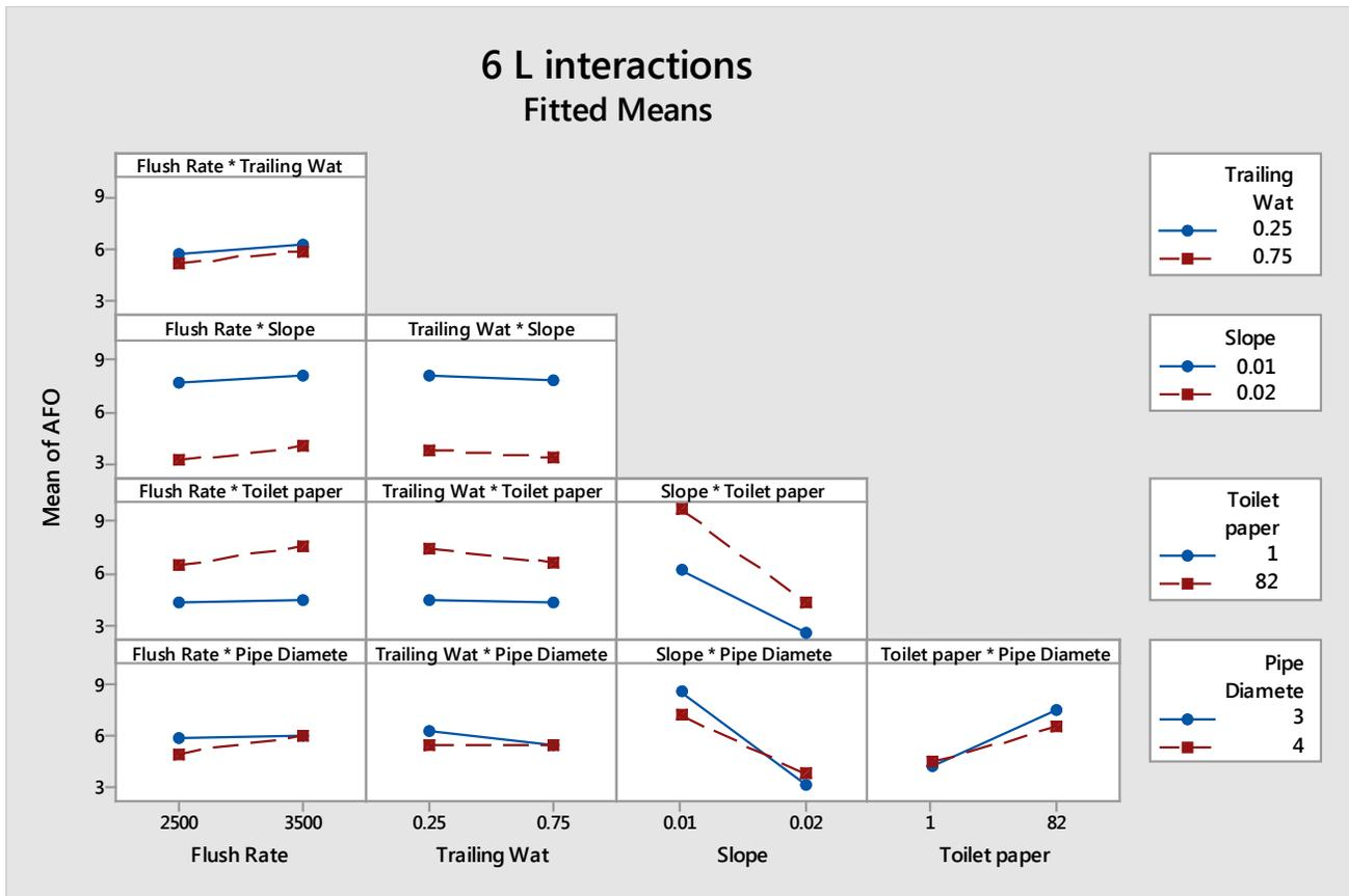
**Table 4-9, General Linear Model: AFO versus Flush Rate, Trailing Water, Slope, Toilet paper, Pipe Diameter**
