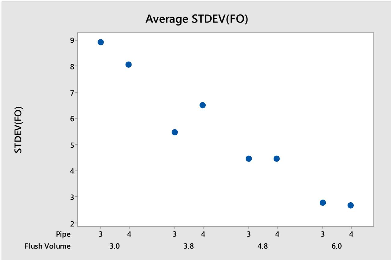
Figure 5-3 below breaks these results down even further by illustrating the influence of toilet paper on STDDEV (FO) results. At every flush volume, variability increases significantly as a result of using high tensile strength toilet paper.
