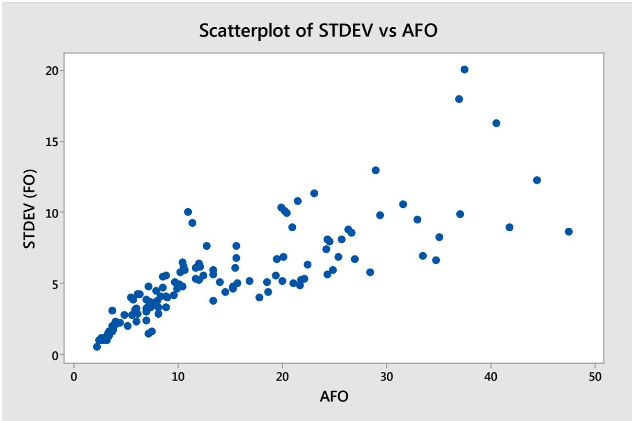
However, considering STDDEV (FO) as a secondary output signal does provide additional insights that further support the primary the findings of the PERC studies. Refer to Figure 5-2 below, which illustrates how standard deviation increases as flush volumes are reduced. It further illustrates the influence of pipe diameter is negligible at the 6.0 Lpf / 1.6 gpf and the 4.8 Lpf / 1.28 gpf flush volumes, and become conflicting at the more chaotic, lower flush volumes.
