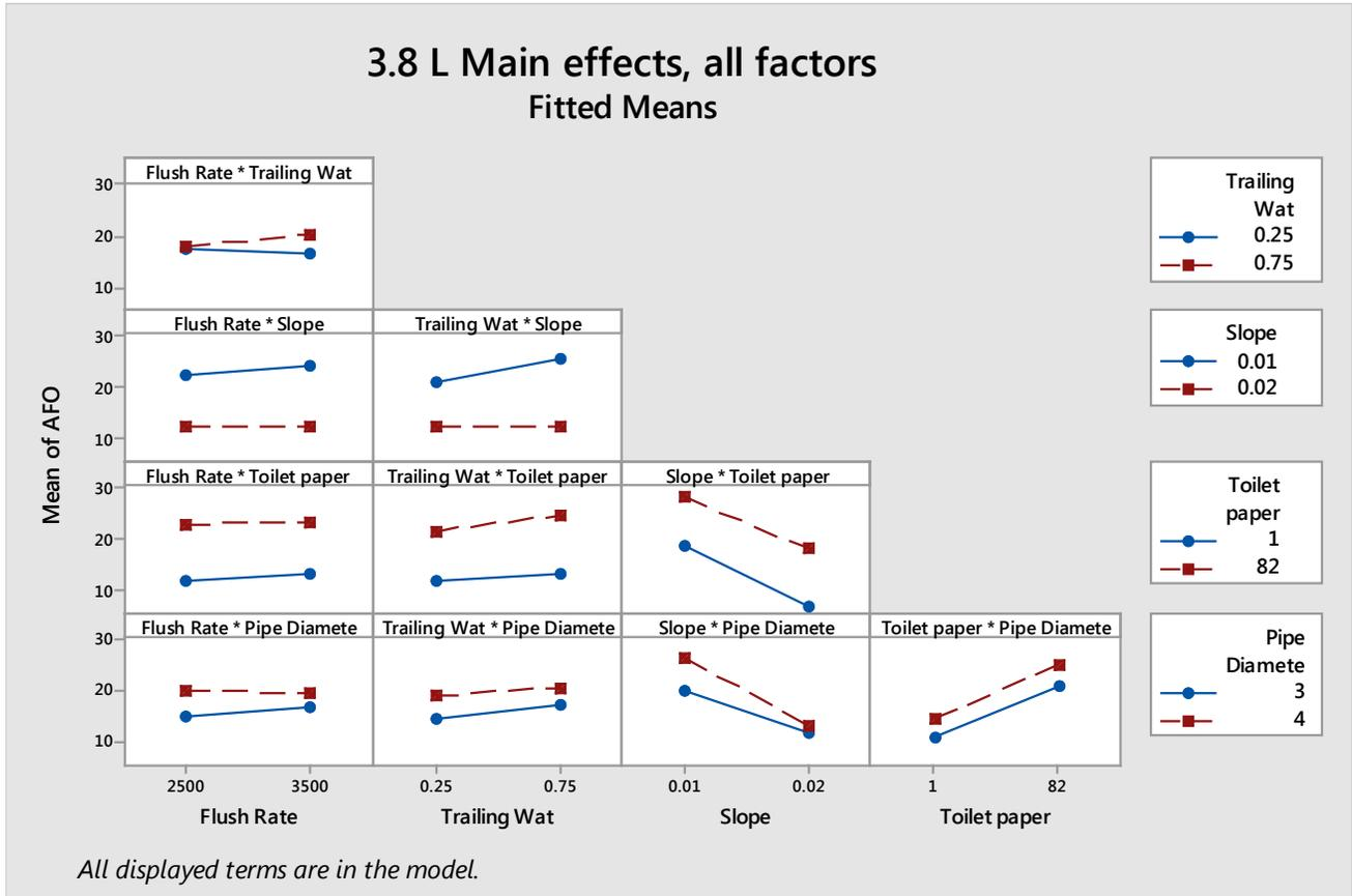
Table 4-11, General Linear Model: AFO versus Flush Rate, Trailing Water, Slope, Toilet Paper, Pipe Diameter
