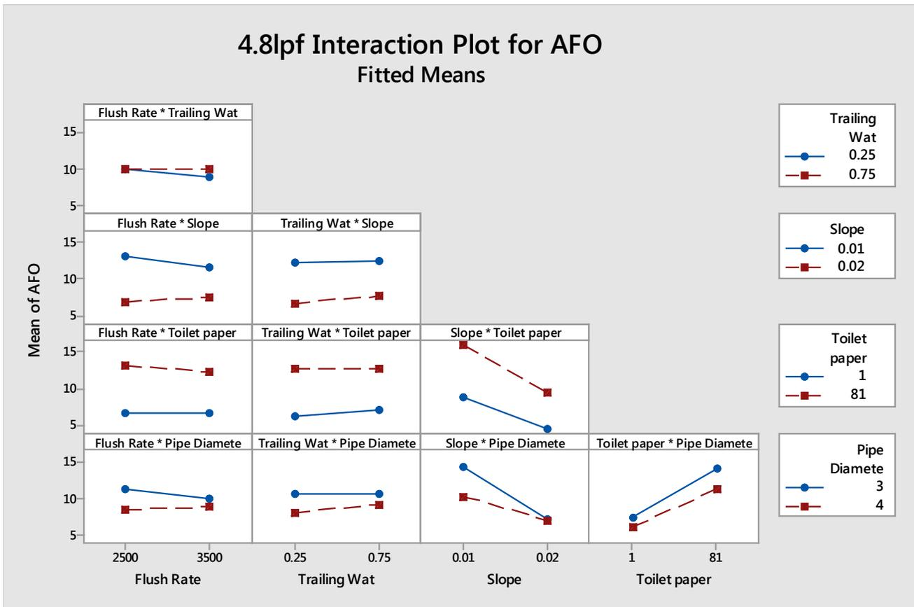
**Table 4-10, General Linear Model: AFO versus Flush Rate, Trailing Water, Slope, Toilet paper, Pipe Diameter**
