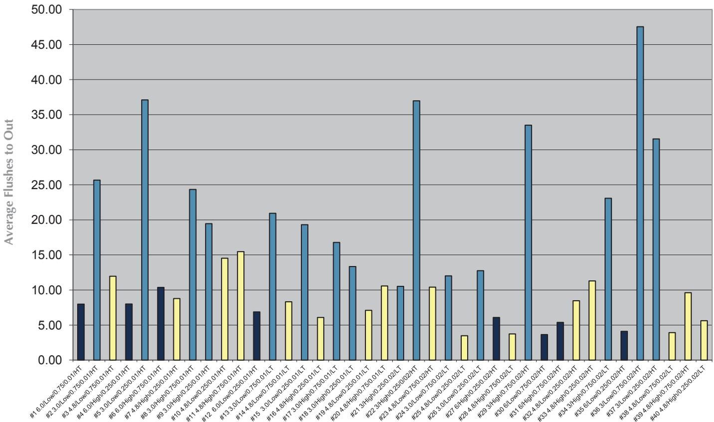
Note: All Test Runs employing 1.6 gallon (6.0 L) injections are shown in dark blue, 1.28 gallon (4.8 L) injection are shown in yellow and 0.8 gallon (3.0 L) injections are shown in light blue.
