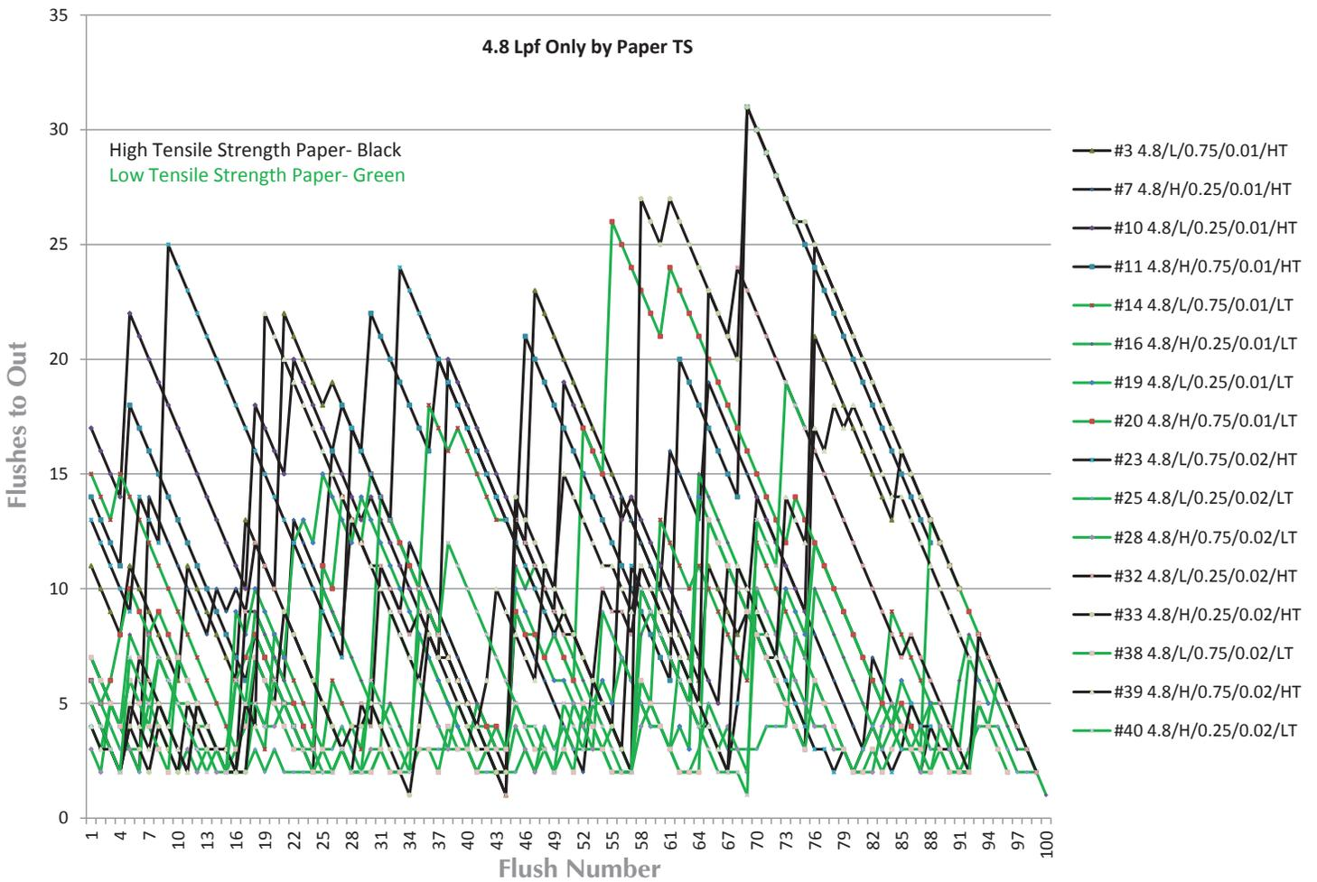
Figure 6-O is a line chart of the same 1.28 gallon (4.8 L) data broken down by toilet paper tensile strength. Past research conducted by ASFlow concluded that selection of toilet paper significantly impacts drainline transport results; thus, the expectation would be to see black over green in this chart, which is clearly evident.
