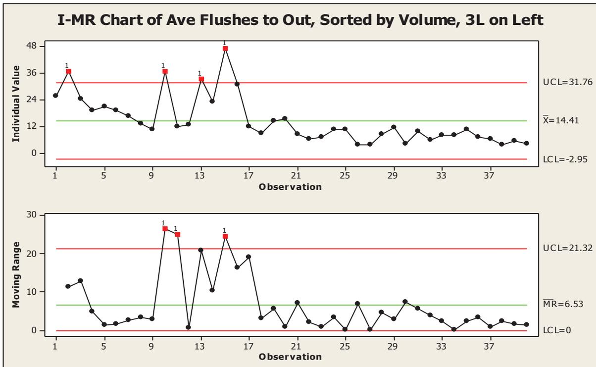
Figure 6-C shows four (4) of the sixteen (16) 0.8 gallon (3.0 L) test runs yielded results that were over the Upper Confidence Limit (UCL) for the data set. This indicates that the results from these tests were random and, accordingly, that the resulting data is being influenced by something other than the test variables. We then ran a Control Chart for the AFO less the data from the 0.8 gallon (3.0 L) Test Runs. The results displayed in Figure 6-D show all data points to be under the UCL.
