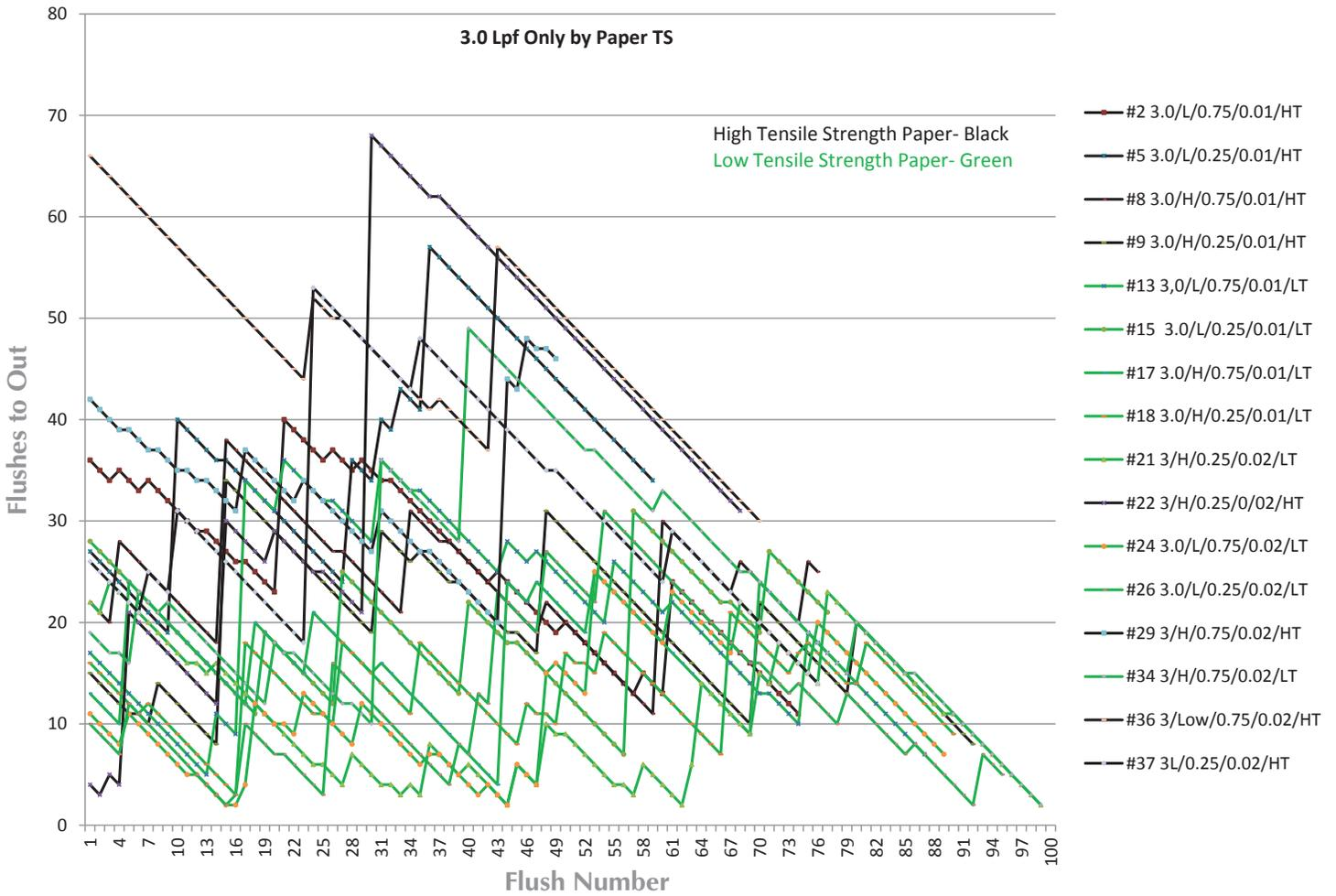
Figure 6-U is a line chart of the 0.8 gallon (3.0 L) data broken down by toilet paper tensile strength. Again, past research conducted by ASFlow concluded that the selection of toilet paper significantly impacts drainline results; thus, the expectation would be to see black over green in this chart, which is clearly evident, even in the chaotic 0.8 gallon (3.0 L) test runs. This result reinforces the importance of paper tensile strength as a significant factor in drainline transport performance.
