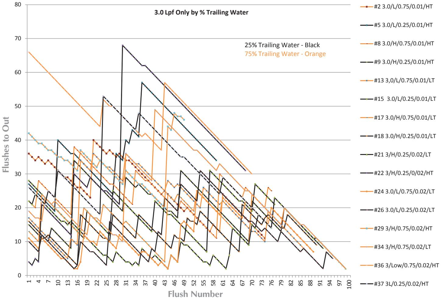
Figure 6-V shows the 0.8 gallon (3.0 L) data broken down by percent trailing water. Once again, based on past research elsewhere that concluded percent trailing water is one of the most significant factors in drainline transport, the expectation would be to see black over orange in this chart. However, consistent with the results in our Main Effects Plots, we cannot determine a difference in the results based on trailing water, and percent trailing water again appears to be non-significant.
