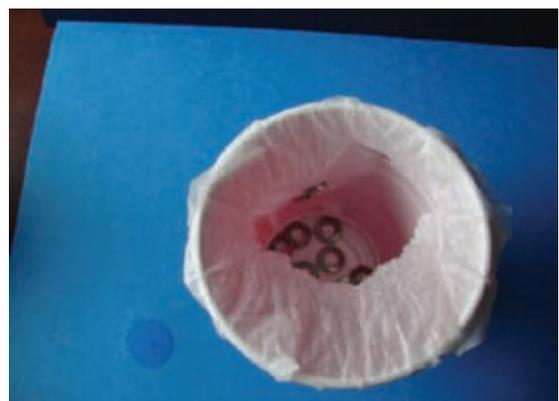
PHOTOS 7-G - TOILET PAPER WET TENSILE STRENGTH TEST
