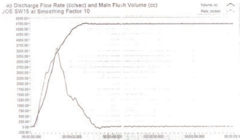
Figure AC-C, above, was generated from an actual 1.28 gpf (4.8 Lpf) toilet. Note that the duration of the flush and the peak flow rate is very similar to the Fast Flush Rate Curve on the bottom of Figure AC-B.
