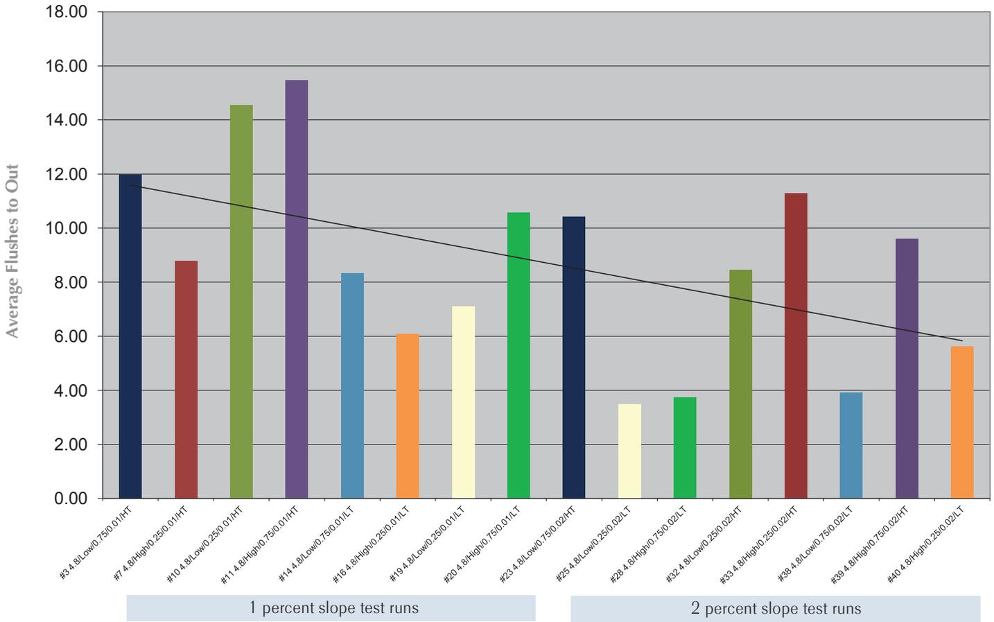
As with the 1.6 gallon (1.6 L) bar chart data, the 1.28 gallon (4.8 L) bar chart in Figure 6-M is also color coded so that test runs at the 1 percent slope and 2 percent slope that embody otherwise identical test variables appear in the same color. Again, the trend line indicates better performance at the 2 percent slope, as expected.
