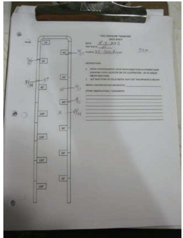
**IMPORTANT** - The number of flushes required for each injection of test media to run the full course of the 135 foot long apparatus and exit was recorded as 'Flushes to Out'. The 'Flushes to Out' values for each injection of test media that exited the apparatus during the 100 cycle Test Run were averaged, yielding the 'Average Flushes to Out' (AFO) data that was used to calculate all results.
