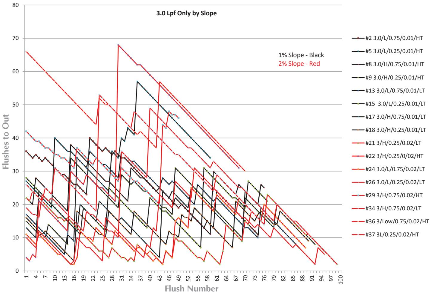
The line chart in Figure 6-T breaks down the 0.8 gallon (3.0 L) data by slope. We would normally expect to see better results (lower AFO) with the 2 percent slope Test Runs, shown in red. The expectation would be to see black over red in the chart. However, consistent with the results shown in Figure 6-S, and per our Main Effects plot on the 0.8 gallon (3.0 L) data (Figure 6-X), we cannot conclude a performance advantage due to slope from this chart.
