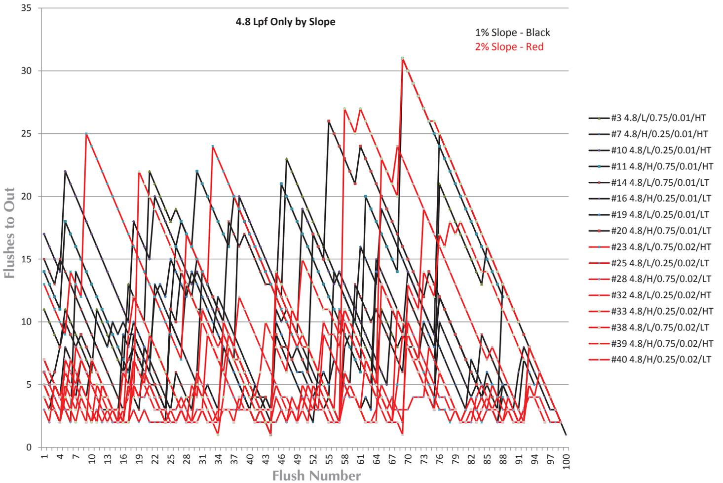
The line chart in Figure 6-N shows the 1.28 gallon (4.8 L) data broken down by slope. We expect to see generally better waste transport results (i.e., lower AFO) with the 2 percent slope Test Runs, shown in red, so the expectation is to see black over red in the chart.
