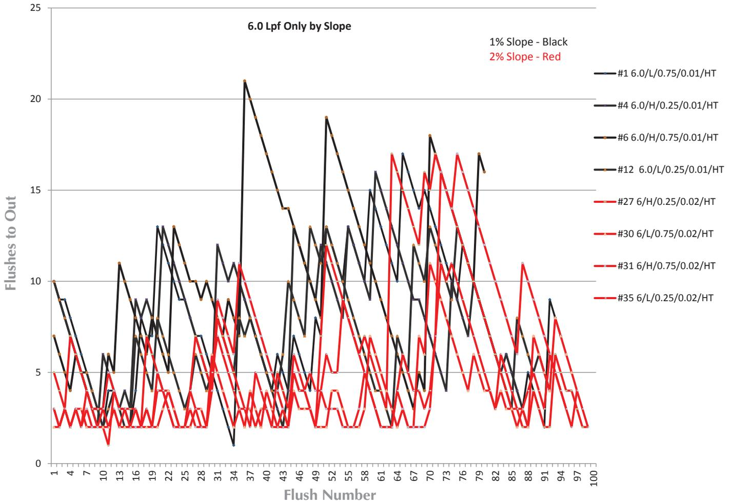
The line chart in Figure 6-1 again breaks down the 1.6 gallon (6.0 L) data by slope. We expect to see better generally results with the 2 percent slope Test Runs, shown in red, so the expectation is to see black over red in the chart as shown.
