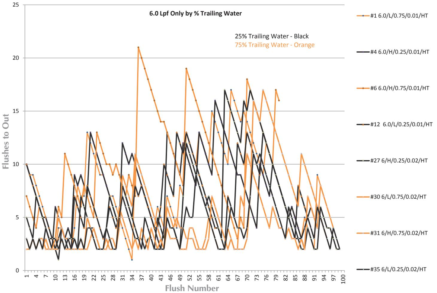
Figure 6-J is a line chart of the same 1.6 gallon (6.0 L) data broken down by percent trailing water. Past research has concluded that percent trailing water is one of the most significant factors in drainline transport; thus, the expectation would be to see black over orange in this chart. However, consistent with the results in our Main Effects Plots, we cannot determine a difference in the results based on trailing water, and percent trailing water again appears to be non-significant.
